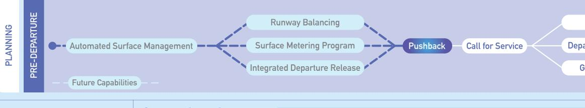
Flight Crew closes door, start the engines, and releases the brakes. Aircraft pushes from the gate into the ramp area.
