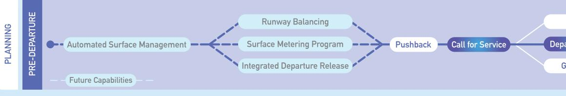
Departure scheduling helps with management of take-off times for aircraft that are expected to join constrained traffic flows along their filed route. This facilitates smooth merging of departures with aircraft that are already airborne, and smooth merging of aircraft through common fixes along their routes.
