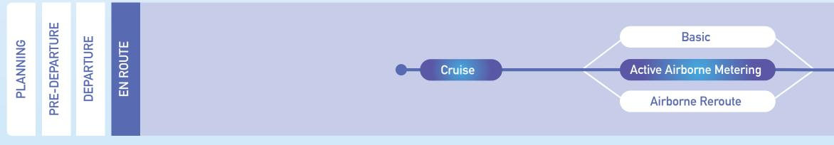
Airborne metering helps ARTCCs manage aircraft merging through congested constraint points along their filed routes. TBFM develops aircraft sequences and times (schedules or timelines) for each adapted constraint point, and applies spacing between specific aircraft pairs rather than uniformly between all aircraft in the flow.
